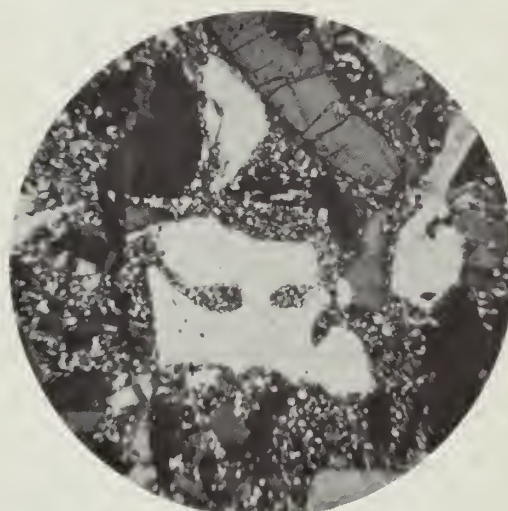
PHOTO 23. A broken plagioclase phenocryst in meta-quartz diorite porphyry north of Big Baldy. Note the prominent zoning as well as the fine mosaic groundmass inset with phenocrysts and fragments of plagioclase, hypersthene quartz and hornblende (crossed nicols).
